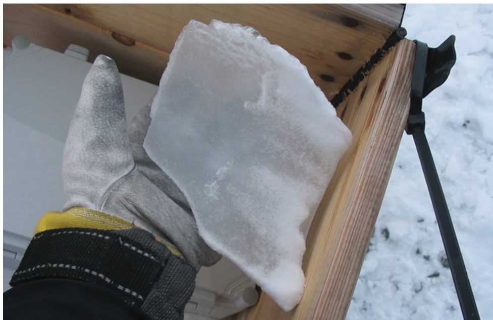
Figure 1: Piece of ice shed from a turbine in Nygårdstjell wind park, Narvik, Norway [5]
