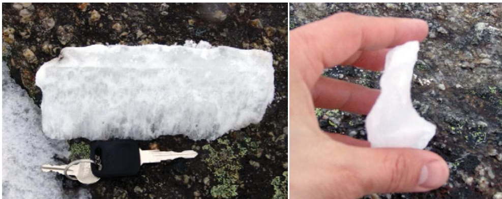
Figure 5: Glaze ice from a wind turbine blade [8]
