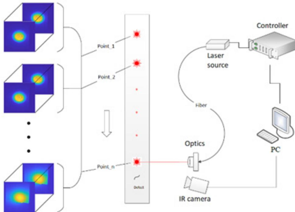
Fig 2. Laser thermography – setup and measurement procedure
