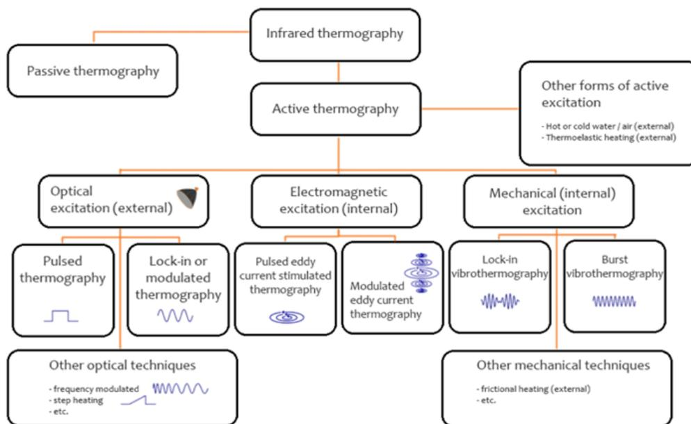
Fig 1. Active thermography – most commonly used techniques [18]
