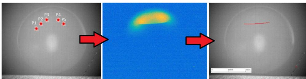
Fig 3. Laser thermography – sequence merging and crack detection [28]
