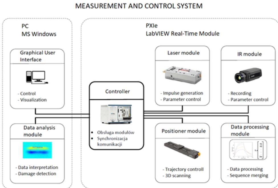
Fig 6. Concept of the laser thermography test system
