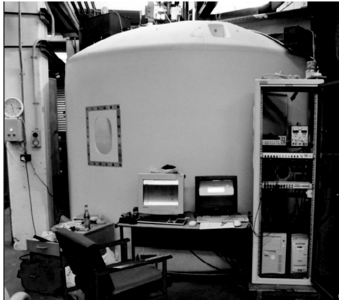
Figure 2 Servohydraulic Slam Testing System.
